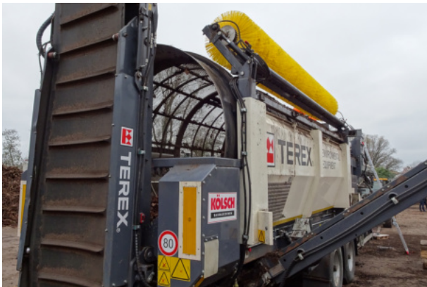
A mobile device for separating the different biomass fractions.
