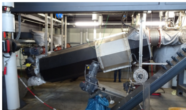
The reactor of the pyrolysis plant. The pyrolysis material is fed through from left to right and quenched at the end.
